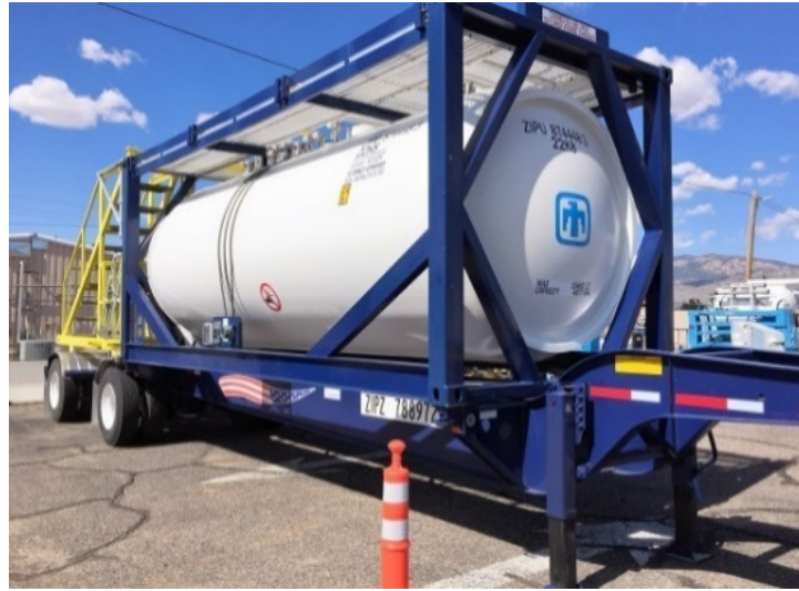
Figure 5. Custom tanker-trailer designed to collect the ~3,000-gallon samples of tight crude and isolate them from air by using water as a piston.
