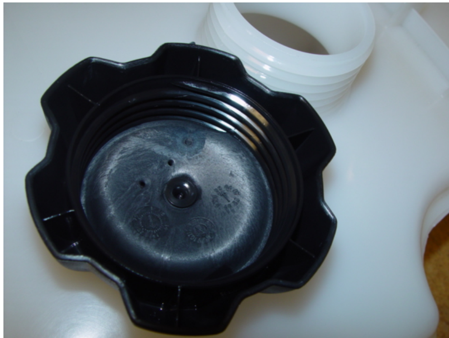
Figure 1b: Fuel cap and seal assembly after a week's submersion into E20. Notice the bulging of the seal due to the extreme swelling of the gasket seal.
