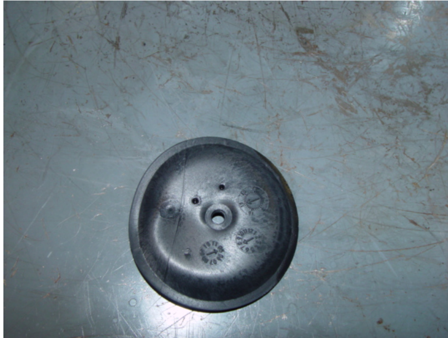
Figure 1c: Fuel seal after a week's submersion into E20. Notice the deformation of the gasket due to the extreme swelling.
