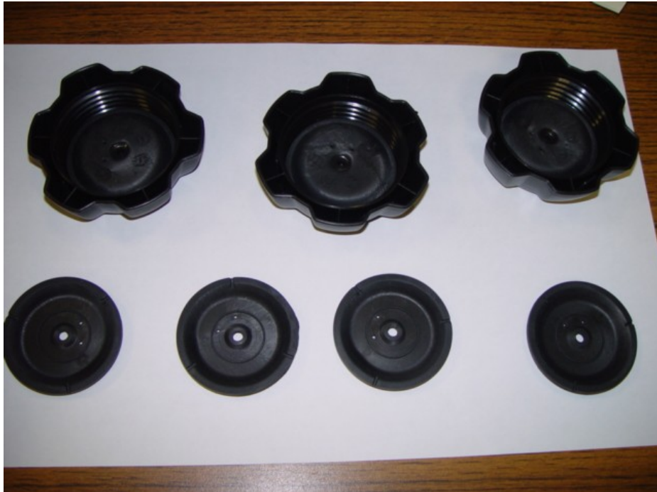
Figure 1a: New and Dry fuel caps and seals prior to fuel submersion testing
