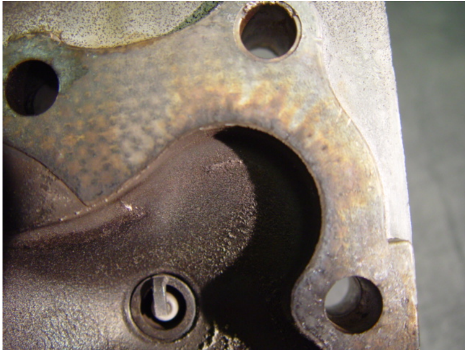
Figure 2a: Cylinder head exhaust blow-by caused by high combustion temperatures.
