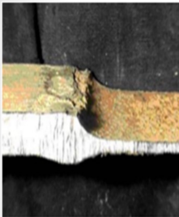
Figure 5: Cross-section of a carbon steel pipe showing preferential corrosion of the pipe with a high residual element content on the right as compared to the low residual pipe section at the left of the weld.
