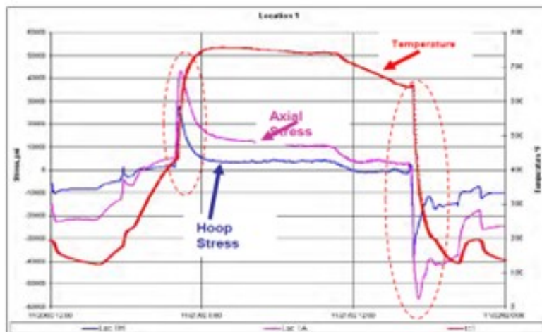
Example of Stresses during Coking cycle
