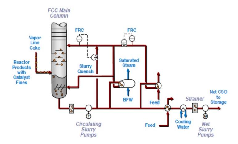
Temperature: From experience, the rate of coke build-up increases greatly when the bottoms temperature is > 700F (370°C). It is recommended to maintain the bottom's temperature below 680°F (360°C) to be on the safe side. Often while processing highly paraffinic feedstock, 660°F (350°C) is a good starting point for MCB temperature and it can be optimized based on monitoring of heat transfer
