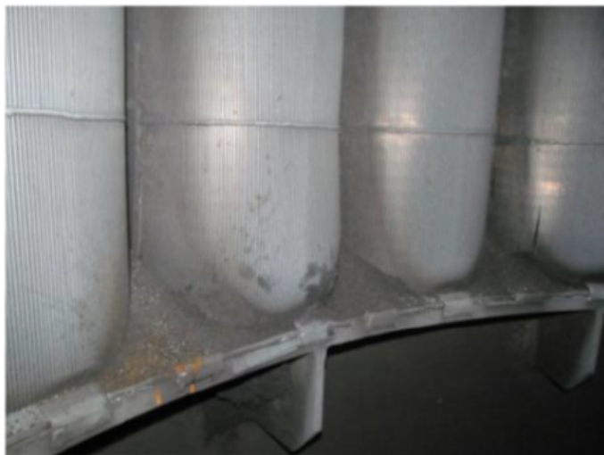
Picture-3(b): Shiny coke between and inside scallops leading to bulging and fish mouth cracks
