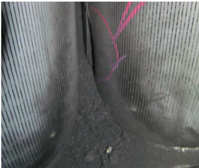
Picture-3(a): Shiny coke between and inside scallops leading to bulging and fish mouth cracks
