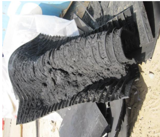
Picture-3(a): Shiny coke between and inside scallops leading to bulging and fish mouth cracks
