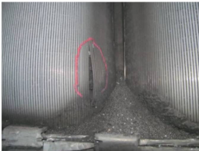
Picture-3(b): Shiny coke between and inside scallops leading to bulging and fish mouth cracks
